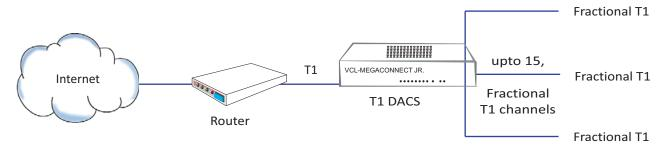
Aggregates upto 15, fractional T1 channels to a single T1
