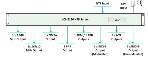
The VCL-2156 is equipped with a highly accurate, low-noise OCXO to provide a high stability, ITU-T G.812, Type II, III compliant holdover clock with better than 12µs accuracy over a 24 hour (5 milliseconds per year) period in the event of unavailability of the GPS / GNSS signal, or GPS / GNSS antenna failure, or a temporary loss of reception in a totally isolated network without any external reference
