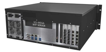
The VCL-Mega NTP Server equipped with a high bandwidth, 16 Core NTP Server engine which is designed to serve up to **One Million NTP requests per second**. A total of 16 x 1G or 10G ports are available in any combination in increments of  $4 \times 1G$  or 10G ports per slot (i.e., a total of  $4 \times$ slots =  $16 \times$ ports). Each 1G port is capable of handling up to 12,000 NTP requests per second and each 10G port is capable of handling up to 120,000 NTP requests per second.
