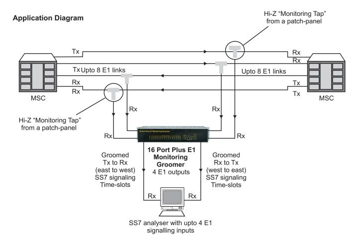
Note: The E1 link is "tapped" through a Hi-Z "Tapping" Port of a DDF Patch Panel.
