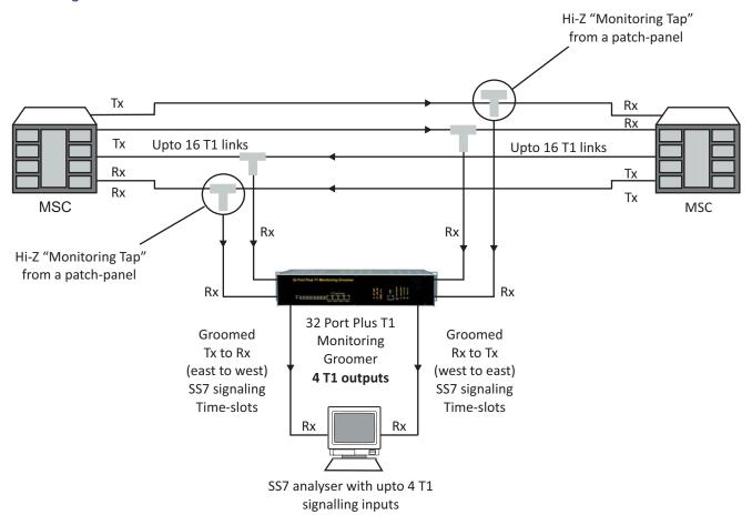
Note: The T1 link is "tapped" through a Hi-Z "Tapping" Port of a DDF Patch Panel.
