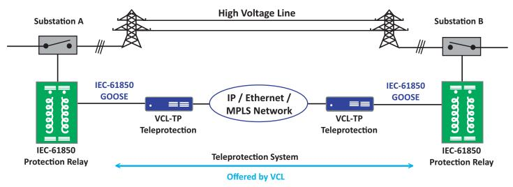
Distance Protection (IEC-61850 GOOSE) over IP / MPLS / Ethernet Network
