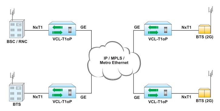
Note: Application illustrates link protection using Spanning Tree Protocol between all nodes.
