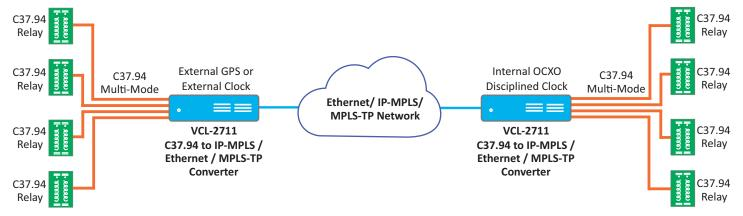
By installing the VCL-2711, the existing C37.94 Protection Relays can be migrated from an SDH / SONET transmission network to an Ethernet / MPLS-TP / IP-MPLS transmission network with no degradation or compromise in the reliability or the performance of the C37.94 interfaces.
