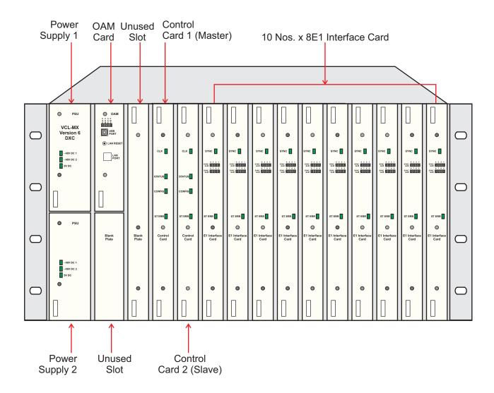
The equipment provides a wide choice of access ports for connecting to and executing management and configuration commands through its OAM Card.
