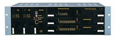
provides the "user" the facility to cross-connect 64Kbps time-slots through a completely "non-blocking" TSI switch, through which the selected SS7 signaling time-slots on the INPUT side E1 Ports can be connected to the OUTPUT side E1 Ports. The equipment provides 16 E1 Ports on the OUTPUT side from where the selected / cross-connected / aggregated SS7 time-slots may be connected to the protocol analysers, test probes, etc.
