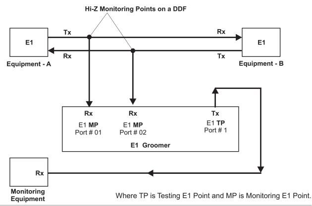
The extreme sensitivity version of the E1 Groomer provides the user with a signal equalizer and a wave-shaper option to handle very low / attenuated E1 input signals.
