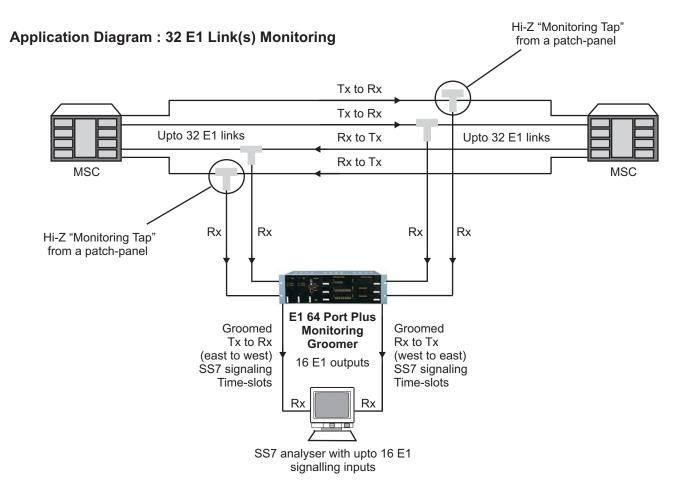
Note: The E1 link is "tapped" through a Hi-Z "Tapping" Port of a DDF Patch Panel.
