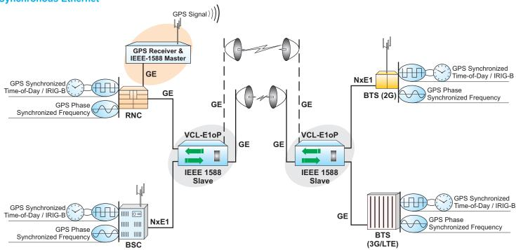
TDM over IP/Ethernet - Distributing E1s, ToD (Time-Of-Day) and Frequency Synchronization over an IP Cloud using IEEE 1588v2\*
